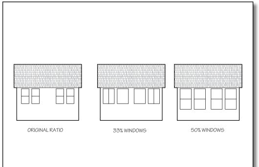
Figure 32—These three drawings show the differences that result from increasing the ratio of openings to solid walls. Noticeably larger ratios produce an incompatible appearance.
