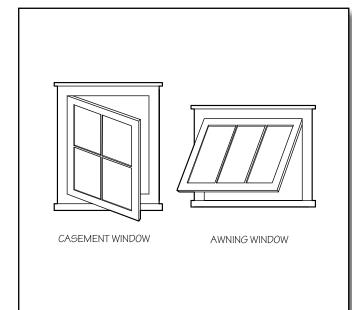
Figure 17—These line drawings show the difference between a side-hinged casement window and a top-hinged awning window.
