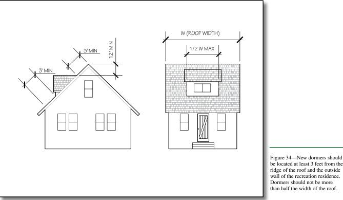
be located at least 3 feet from the ridge of the roof and the outside wall of the recreation residence. Dormers should not be more than half the width of the roof.
